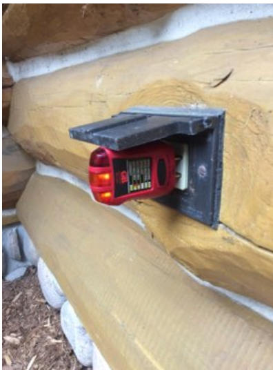
Exterior receptacles tested and functioned properly
