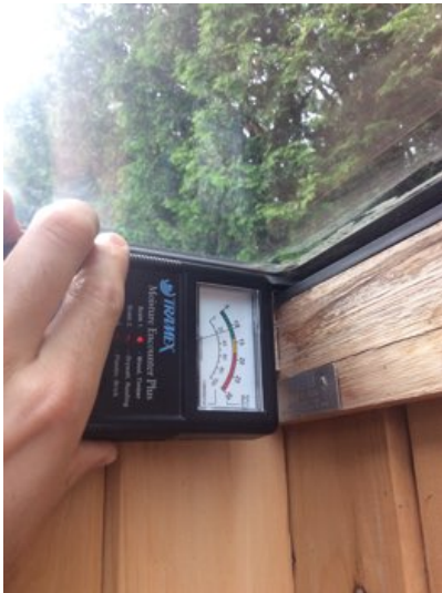
Staining at the kitchen skylight window tested dry at time of inspection with moisture meter
